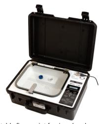
A fully portable fingerprint fuming chamber mounted within a rugged weather-proof case, the MVC lite retains all the features of a full sized fuming chamber and can be used for the development of latent fingerprints using both cyanoacrylate and PolyCyano UV, the cyanoacrylate/fluorescent stain that eliminates the need for subsequent chemical staining.
