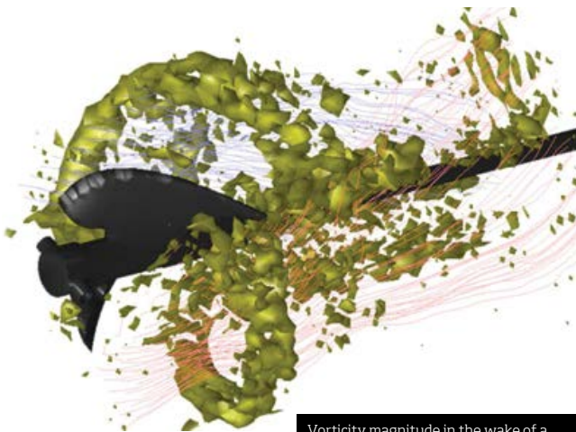
Vorticity magnitude in the wake of a model ship propeller with streamlines.
